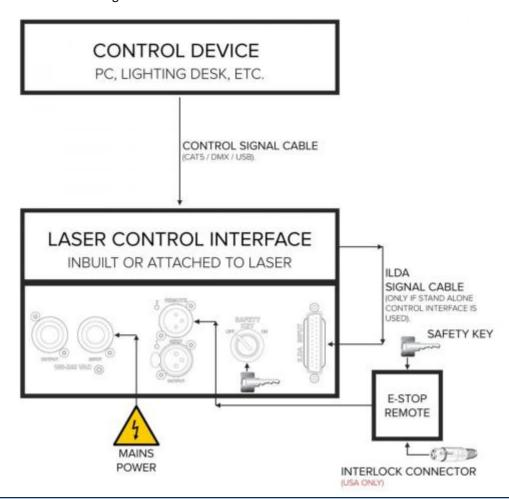
\* Both E-STOP Remote safety key and laser system safety key must be inserted and switched to ON position in order to disable the interlock.
