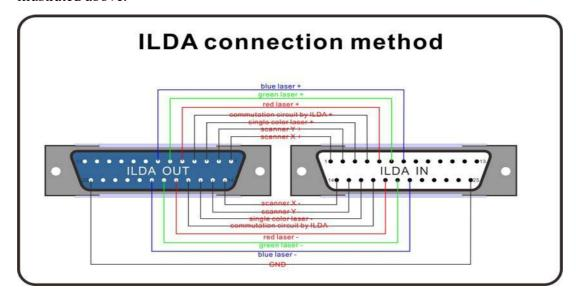
ILDA control signal connection method:
